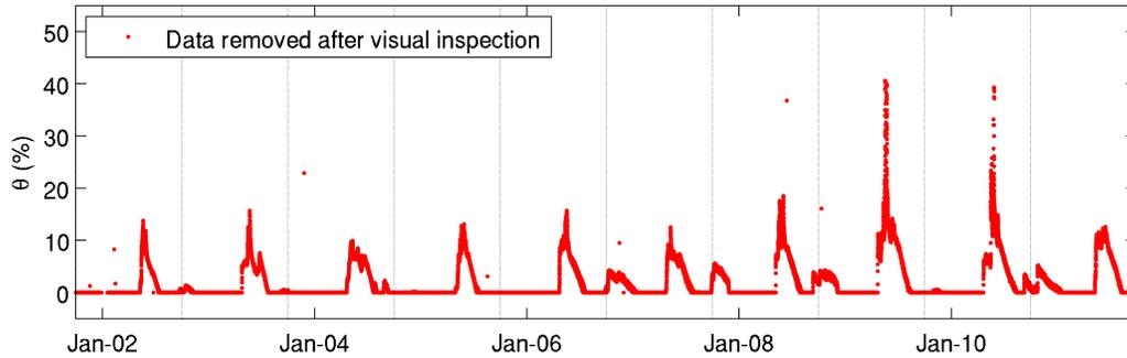
Figure A.4: Soil water content data from the Big Sandy Opening, WY SNOTEL site. All data from this sensor were excluded because the majority of data reported is at 0 % water content. The sensor response may have been out of the range of the calibration equation used by NRCS. Dashed vertical lines are plotted at the start of each water year (Oct 1).
